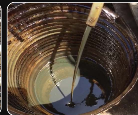
Heavy hydrocarbons removed from MDEA
